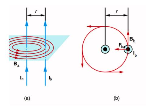
The current in the conductor 'a' produces the same magnetic field at all points along the conductor 'b' and its magnitude is given by
